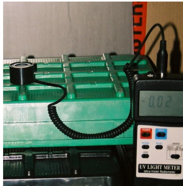
Figure 3. UV light meter as used in the base line experiment to determine the effect of spray boom velocity and distance from the source on the dose rate received.
