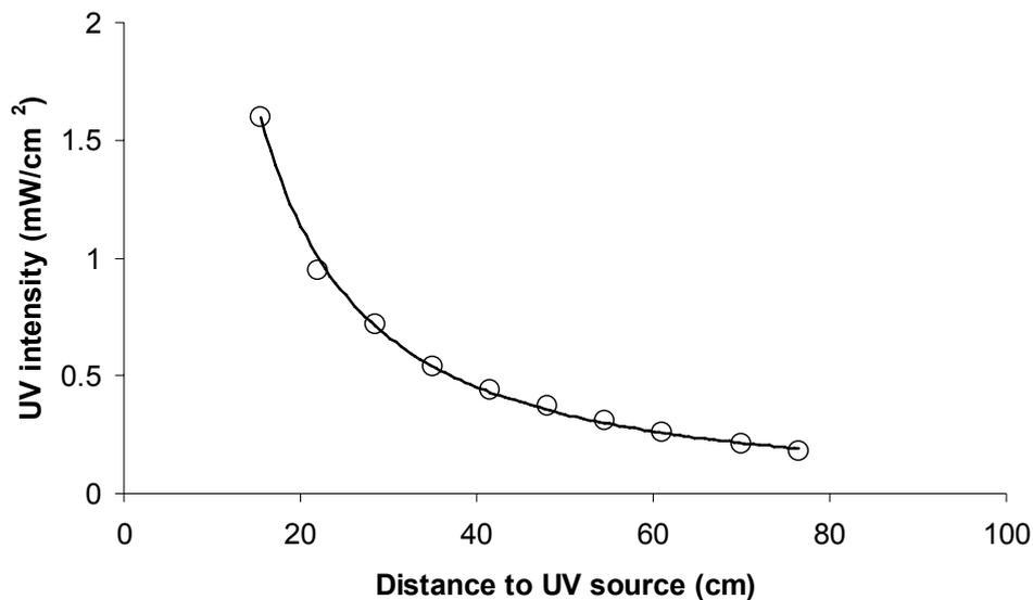
Figure 5. Effect of “distance from the source” on UV intensity as measured in the base line experiment using a Lutron UVC-254 UV light meter. The regression line is mathematically described by Equation 2.
