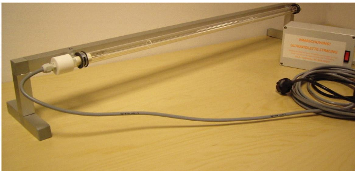
Figure 2. The 75 Watt UV source (Philips TUV 64T5 4P SE) as used in the experiment.
